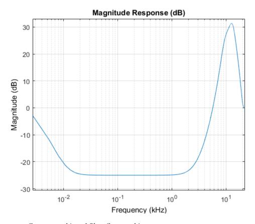
Construct a biquad filter System object.
