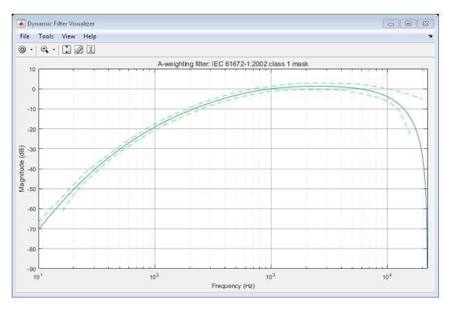
Create a spectrum analyzer to visualize the original audio signal and the audio signal after frequency-weighted filtering.
