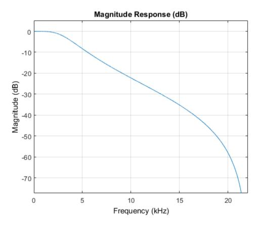
Construct a biquad filter System object.
