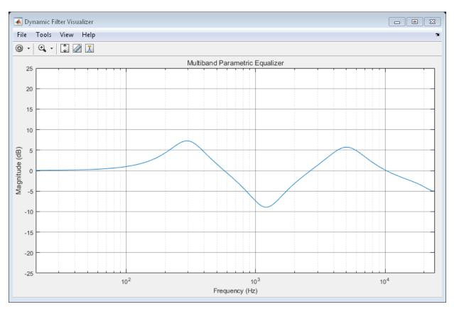
Play the equalized audio signal. Update the peak gains of your equalizer band to hear the effect of the equalizer and visualize the changing magnitude response.
