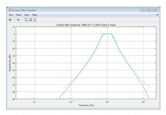
Get a vector of valid center frequencies, given the center frequency of octFilt. Create an octave filter bank using the valid center frequencies.
