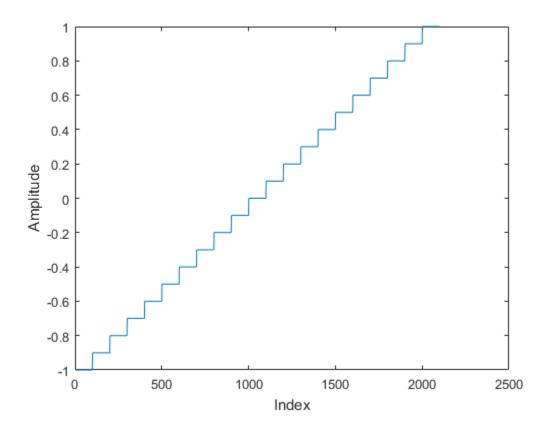
Create a wavetable synthesizer, waveSynth, to generate a staircase wave using the single-cycle waveform. Specify a frequency of 10 Hz.
