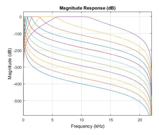
Visualize the octave filter bank with a logarithmic frequency scale. The logarithmic frequency scale makes the center frequencies appear evenly distributed.
