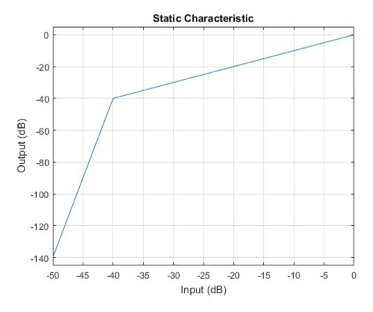
Set up the scope to visualize the signal before and after dynamic range expansion.
