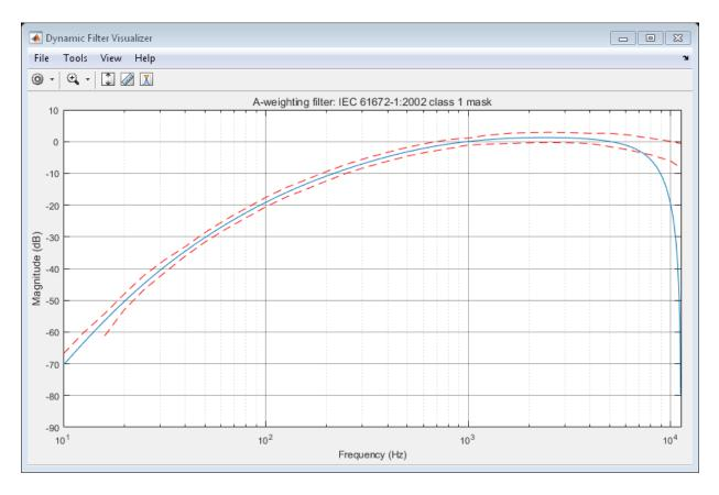
Change your A-weighting filter sample rate to 44.1 kHz. Verify that the filter is standard compliant and visualize the filter design.
